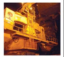
the world. The project harnessed the in-house capability of JSPL's heavy machinery division in Raipur, which provided technological equipment's and manufactured the biggest Ladle Turret for the Angul Plant.
