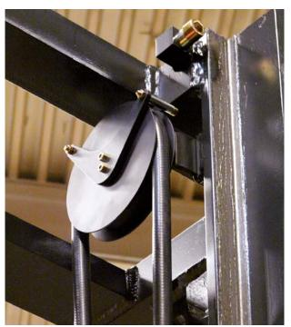
Energy and signal cables up to 14 metres in length are guided in the hoist frame by guide rollers, and move every time the mast is raised or lowered. (Source: igus GmbH)
