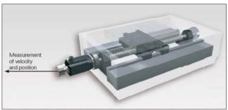
Figure 2: Position feedback control with a recirculating ball screw and a rotary encoder in semiclosed-loop mode
