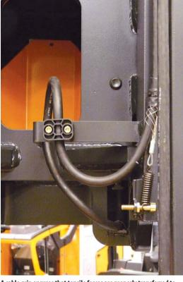
A cable grip ensures that tensile forces are properly transferred to the cable. (Source: iqus GmbH)
