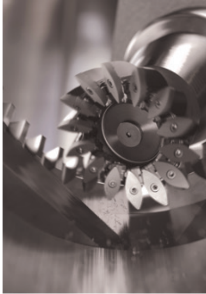
Power skiving, with tools like CoroMill 180 indexable power skiving cutter, enables all machining to be carried out in one single set-up
