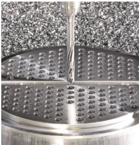
Figure 4: Helical flutes with variable helix angle in a LOGIQCAM drill body improve the dynamic behavior of the drill and increase the drilling depth to eight drill diameters.
