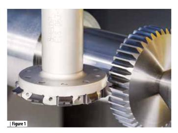
TECHNOLOGICAL PROCESSES DEVELOPED FOR THESE MACHINES ARE ORIENTED TO MAXIMIZE MACHINING OPERATION FOR ONE-SETUP MANUFACTURING, CREATING A NEW SOURCE FOR MORE ACCURATE AND PRODUCTIVE MANUFACTURING. MILLING GEARS AND SPLINES IS ONE OF THE OPERATIONS SUITABLE FOR PERFORMING ON THE NEW MACHINES.
