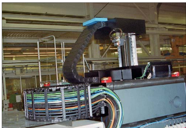
Saving space: the X-axis of the energy chain lies on the upper machine cover.
