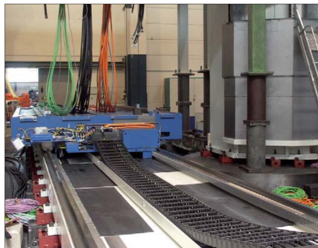
Holding chainflex®-cables in e-chains® for motion-control applications.
