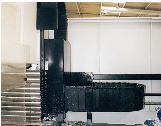
igus® E2 e-tubes, upright and rotated by 90° in the chip area.
