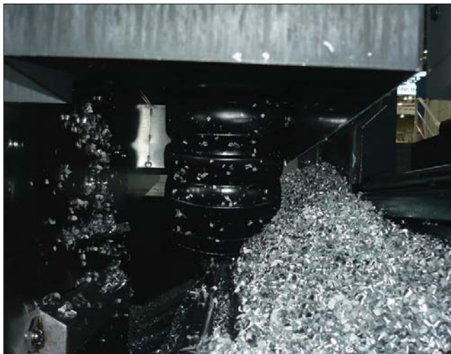
igus® RX e-tube – ideal in the direct chip area, IP protection class 40.
