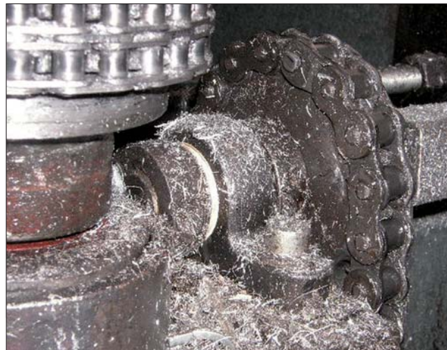
Dry-running igubal® plastic spherical bearings – no chip adhesion.
