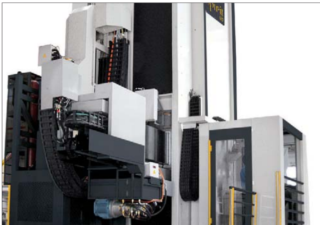
Several e-chains® and chainflex® cables in various installation methods.
