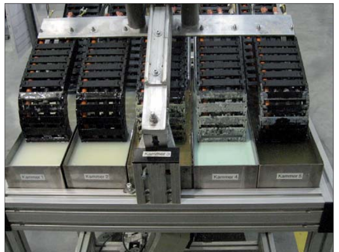
Media resistance testing on chainflex® cables
