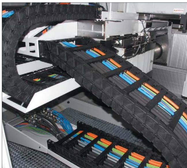
Combined motion with an igus® E6 readychain®.
