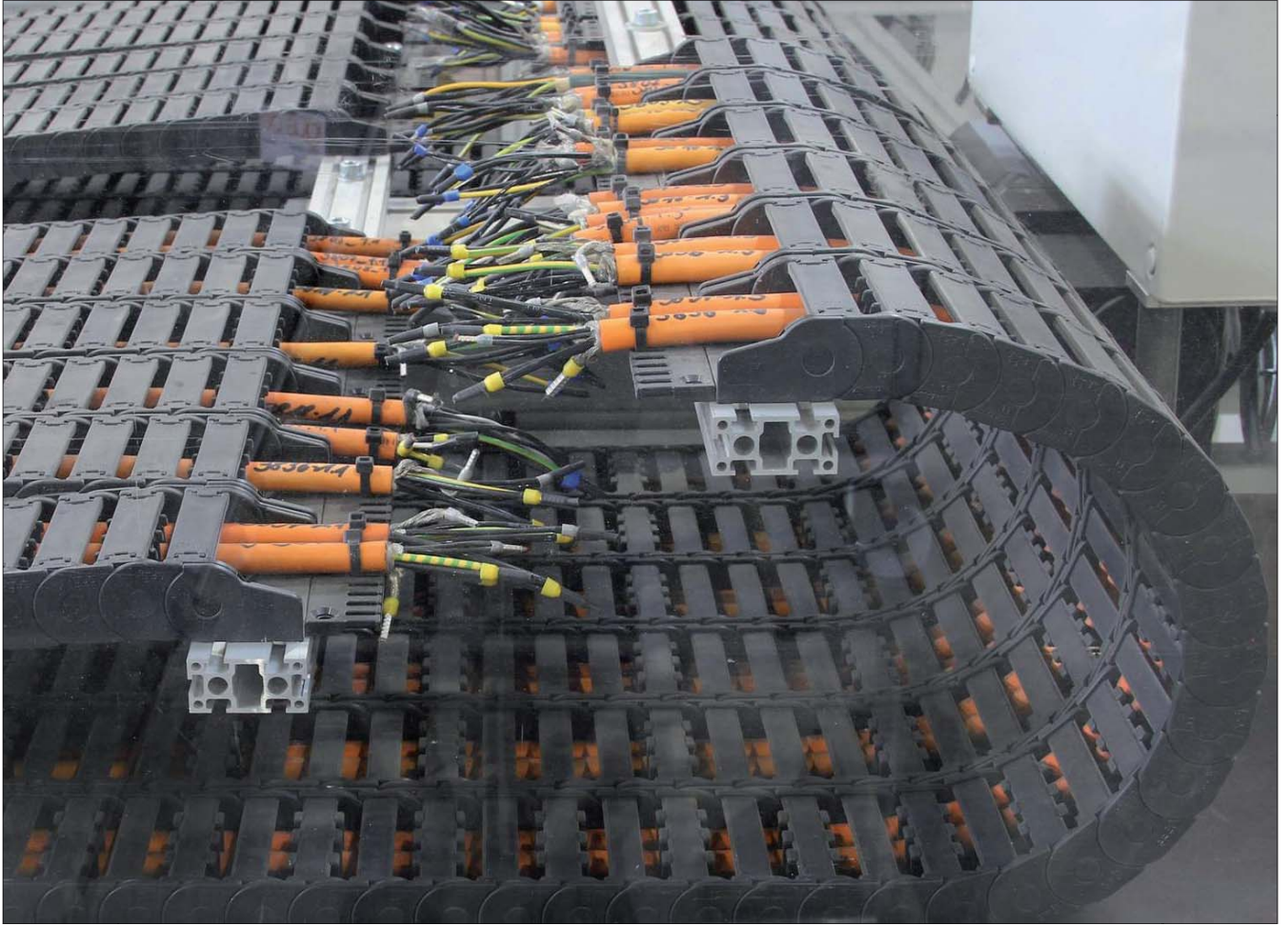
Cable service life test at the igus® lab, Cologne.
