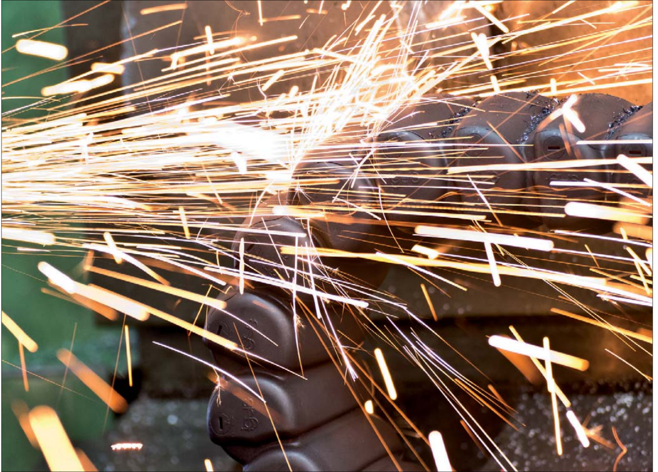
Heat-resistant against 850°C hot chips: igus® RX e-tube as HT configuration (optional).
