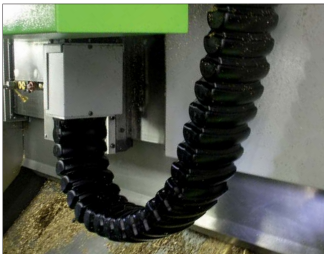
Brass chips and oil/coolant – igus® RX e-tube protects reliably.
