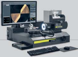
»pomBasic« Compact solution for a universal tool inspection
