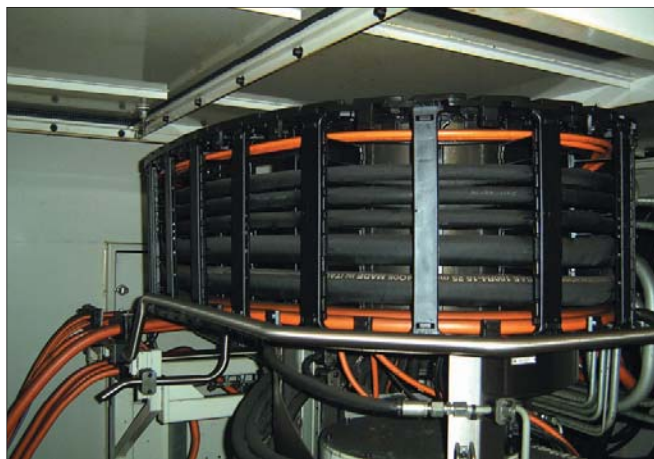
e-chain® E6 in a CNC grinder: its low weight supports particularly smooth motions.
