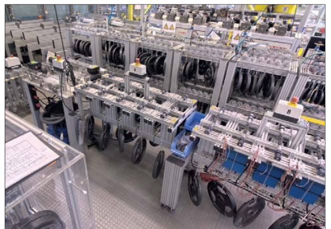
Tribology testing in the plain bearing lab, igus ® Cologne.
