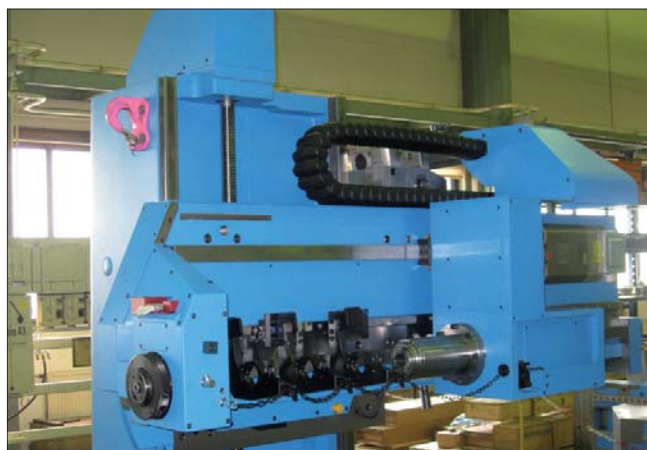
RX e-tube: problem-solver on the machine tool in the chip area.
