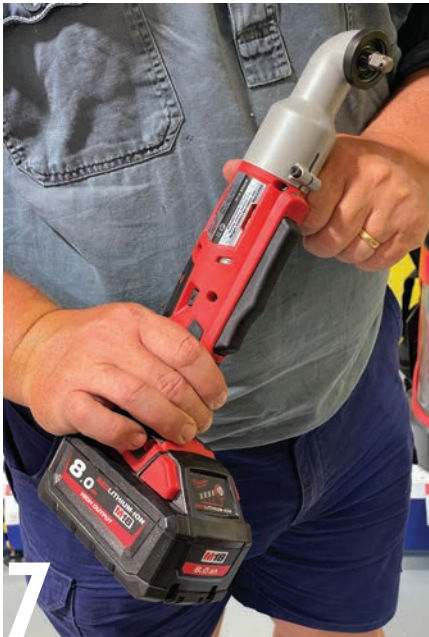
7 This Milwaukee right-angle 3/8" drive impact wrench caught our eye, and would be ideal for working in confined spaces. With two torque settings of 40 or 60Nm, it is never going to undo wheelnuts or remove seeding points, but might just fit the bill for a specialist application. Priced at $300 for the skin.
