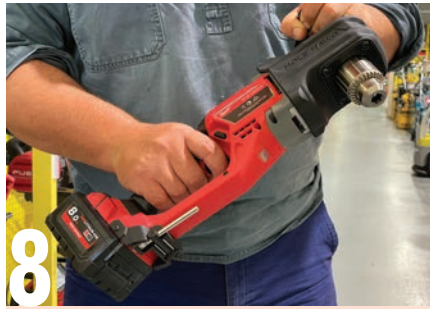
8 If working in tight spaces is your thing, the Milwaukee "Hole Hawg" right-angled drill might be a little more useful. The 18V unit is fitted with a 13mm chuck, with the key stored on the tool itself. It features a max speed of 1500rpm and 11 torque settings for driving (up to 43Nm), and costs around $450 for the skin. Others are made by Dewalt ($599 skin) and Makita ($669 skin). There is a cheaper 18V Milwaukee version available for $300, or a 12V unit for $149, both as skins with 10mm chuck.
