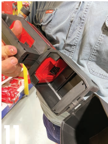
11 This Milwaukee transfer pump caught our eye ($359 for the skin). It can shift 30L per minute to a head of 23m and is self-priming with a suction lift of 5.5m. The positive displacement pump has a clear window over the pump impeller (top), and the battery fits into a splash-proof compartment for additional protection (bottom). Apparently it can shift up to 900L off one 5Ah battery charge. However the unit is only rated for water; how handy would it be if it was rated for fuel and oil?
