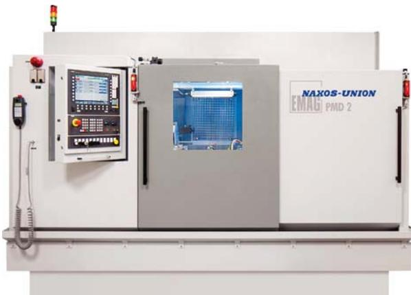
**Compact design:** The enclosure also contains the electrical cabinet and the energy container. Equipping the machine with an automatic loading system is no problem.
