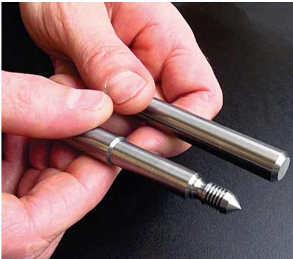
**The WireDress technology allows free geometries and intricate contours with internal radii of 0.05 millimeters and external radii of 0.2 millimeters.**
