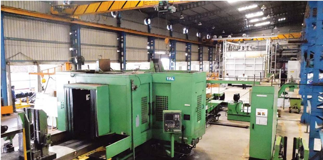
Rejection of parts at the TAL 1 machine was eliminated by adding Air / Coolant blast during tool change to ensure chip removal between Boring Bar and Spindle Face.
