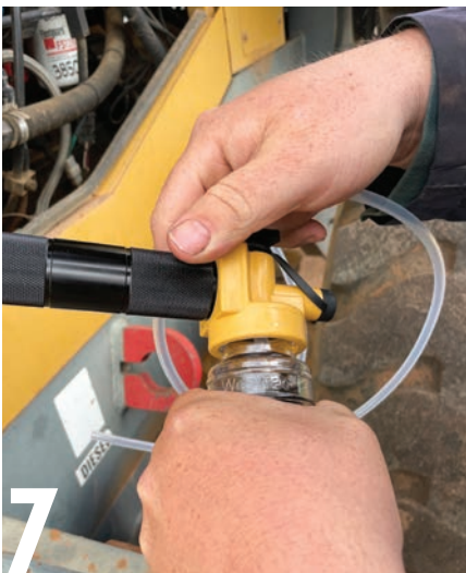
7 Remove the solid cap from the sample bottle and attach securely to the vacuum pump, taking care not to contaminate the inside of the bottle.
