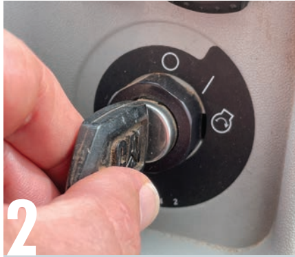
2 To take an accurate, representative sample, it is imperative the machine is brought to operating temperature. In the case of an engine oil sample, simply start the engine and bring to working temperature to ensure the oil is correctly mixed. For another reservoir such as a final drive, transmission, differential or hydraulic system it will be necessary to operate the machine to ensure oil is well mixed.
