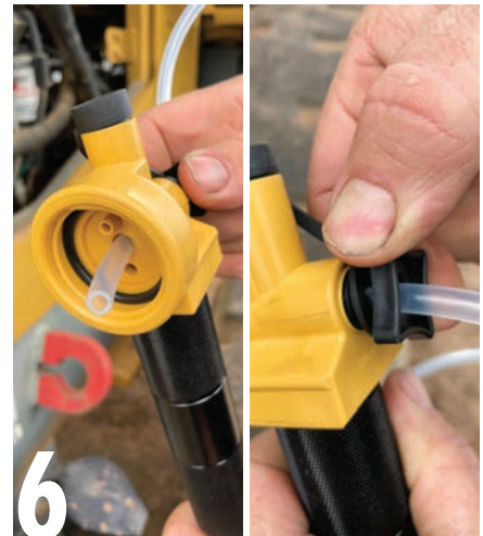
6 Insert the trimmed end of the tube into the vacuum pump so that the end protrudes by about 25mm (left). Now tighten the collar nut to secure the tube (right).
