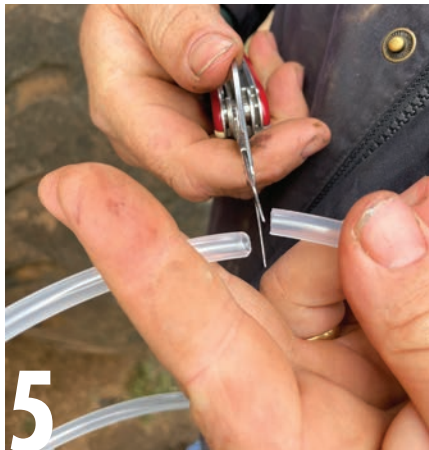
5 Now cut the tube to length allowing additional tube length for the vacuum pump to be conveniently operated. Note that the longer the tube, the more difficult it will be to draw a sample. Make sure the tool used to trim the tube is clean and doesn't contaminate the cut.
