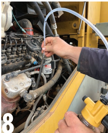
8 Insert the end of the sample tube into the dipstick tube, taking care not to brush the end against anything than may contaminate the sample. Make sure the tube is inserted to the marked line. It may pay to have a helper hold it in place. Alternatively, secure with a piece of tape.
