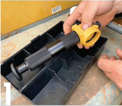
1 It is most likely a vacuum pump will be needed for the majority of sampling jobs on farm. This screws to the top of the sample jar and is used to draw a sample of oil through a tube and into the jar. It costs about $40. While samples have been taken from the oil stream when draining a sump during an oil change, it is not worth the effort due to the difficulty in obtaining an accurate sample (and the ensuing mess!).
