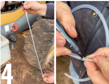
4 Holding the sample tube alongside the dipstick, mark the length of the dipstick on the tube with a felt tip pen. This will ensure the sample tube draws oil from the around the level of the dipstick. If the tube is inserted too far into the sump it will draw a sample from the base of the oil pan which may not be representative. For other compartments without a dipstick (for example final drives, differentials) ensure the compartment is level and the tube is inserted roughly half-way into the oil.
