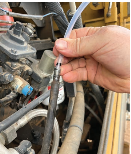
6 Insert the trimmed end of the tube into the vacuum pump so that the end protrudes by about 25mm (left). Now tighten the collar nut to secure the tube (right).
