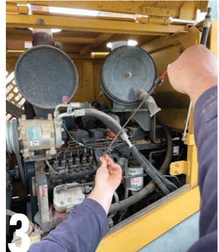
3 With the engine at operating temperature, switch off and make sure the unit is in park. Withdraw the dipstick and wipe off any excess oil.
