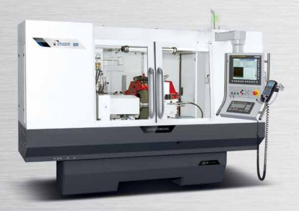
If versatility is your concern, then the S31 is the ideal machine for you. It is designed for producing medium-sized workpieces in individual, small batch and mass production. Its Granitan® S103 mineral casting machine bed largely equalizes temporary temperature fluctuations. The swiveling wheelhead allows you to externally, internally and face grind workpieces in a single clamping – with a high-resolution B-axis of 0.0001 deg.
