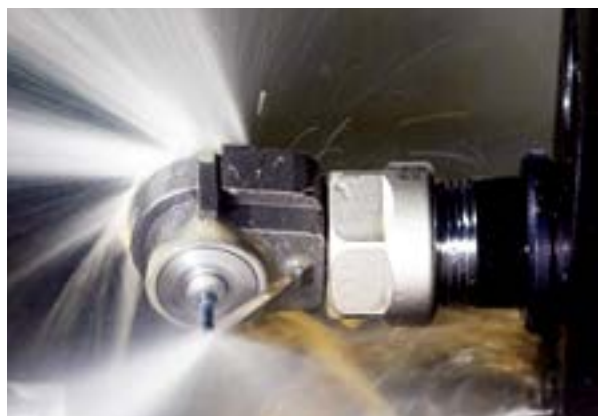
A Micro 90 coolant-driven high-speed compact spindle ensures extremely high rotating velocities.
