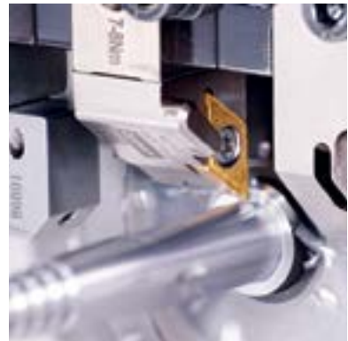
A NEOSWISS turning tool carries a quick-change head with indexable insert.
