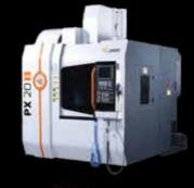
PX Series INVU CNC Vertical Machining Centers
