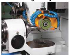
mills/form tools. Electrical elements are designed to reduce the electromagnetic interference & reduced emissions to make the machine environment friendly. Types of tools manufactured and reground include end mills, ball nose, CR end mill, drill & step drill, form tools, gun drill, inserts, thread mill, taps, form radial cutter, etc.
