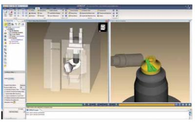
VERICUT CNC machine simulation, verification and optimization software simulates all types of CNC machining. VERICUT Force™ is a physics-based optimization method that determines the maximum reliable feed rate for a given cutting condition based on the following three factors: maximum chip thickness, maximum allowable feed rate, and force on the cutter. The software operates independently, but can also be integrated with leading CAM systems.
