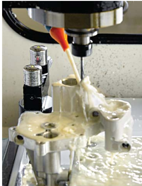
The Renishaw NC4 system is used to prevent damage caused by damaged tools to very expensive parts – eliminating resultant scrap, re-machining and wasted time.
