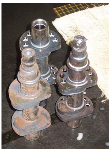
The Desmodromic camshaft is not conventional, and has been designed with special 'lifting ramps'
