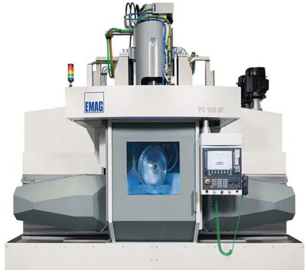
Blisk machining on an Emag PO 900 BF
