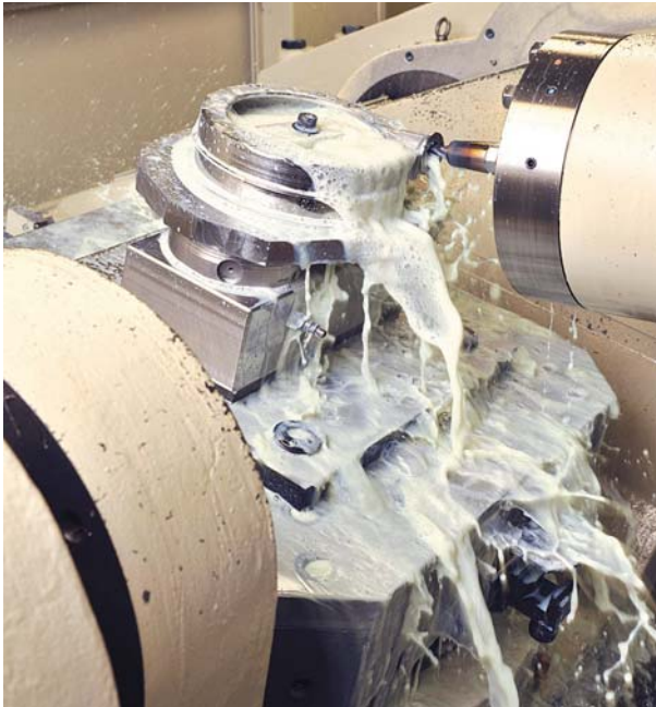
These latest generation hard metal machining systems, which also include the latest tool/spindle interfaces, can handle up to 35,000 inch-pounds of tool taper moment loads to accommodate long tools cutting highly resilient materials.
