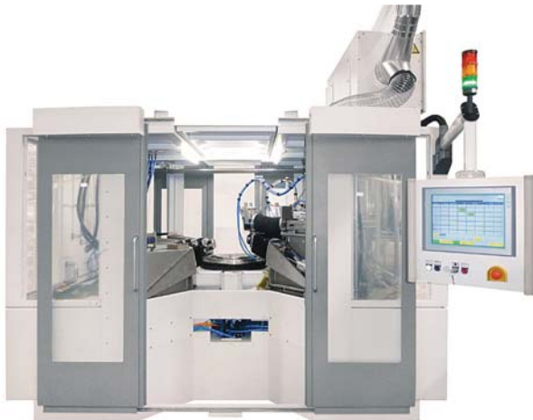
Emag ECM machine for the multi-station machining of turbine disks
